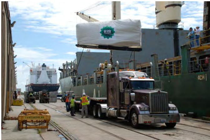
Wind turbine nacelles are discharged directly from ship to truck at the Port of Morehead City, NC.
