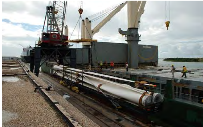
Four wind turbine blades in a specialized blade cage system are discharged from the PAC ADARA by NC Ports shore crane.
